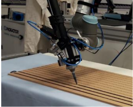
Robotic System for Adhesive Application and Joint Sealing
