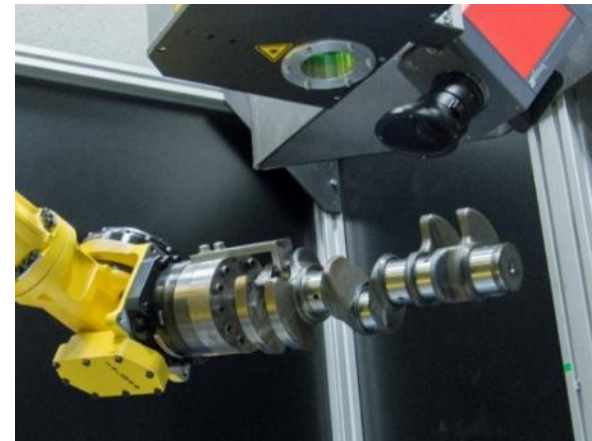
Crack Detection by Thermography
